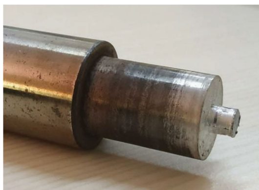
Fig. 1 Photograph and the dimension of FSP tool (all dimensions are in mm)
